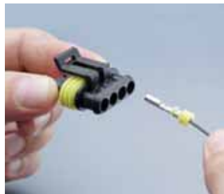
[7] Insert each terminal/wire into universal plug connector.
