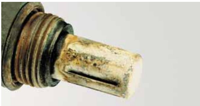
Coolant / anti-freeze contamination
