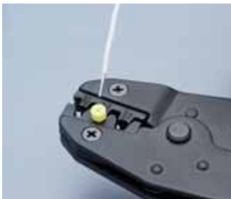
[5] Insert wire into terminal (pass through the closing rubber).
