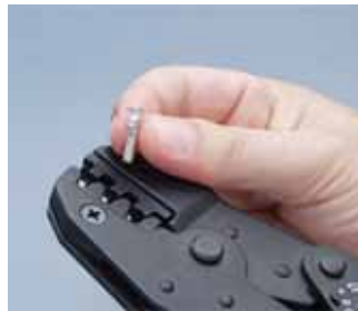
[3] Insert terminal into crimp tool with open part in crimp tool cavity.
