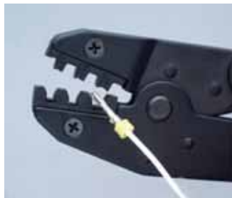
[6] Press crimp tool to lock wire in terminal.
