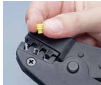
[4] Partially close crimp tool to hold terminal in place and insert closing rubber with smaller diameter.
