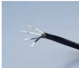
[2] Remove the end insulation of each wire.
