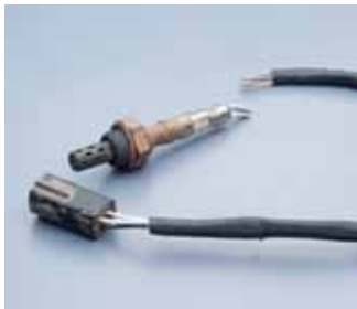
[1] Cut wires off close to body of used sensor.
